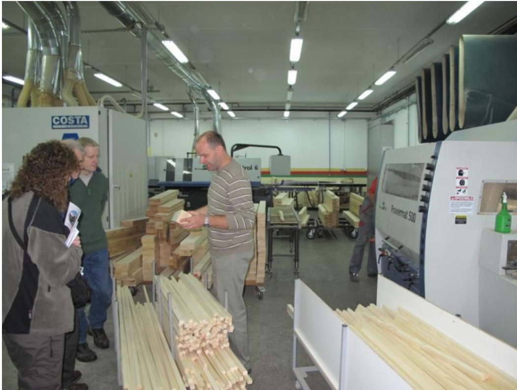
Plate 11. Part of the window production facility with mouldings produced by CNC machine.
